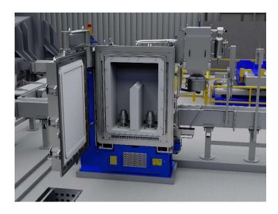
The Hycast® I-60 SIR sets the benchmark for the in-line refining of molten aluminium at casting centers. The unit has one reactor chamber with a baffle and two rotors, that can handle up to 70 t/hour.
